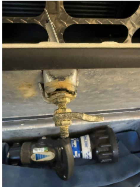
All corroded latches and corroded gas struts need to be replaced.
