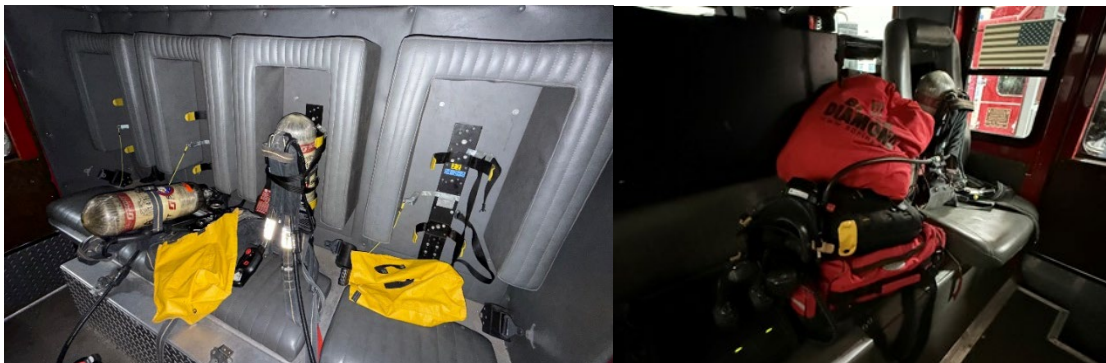
This unstrained SCBA and equipment could injure or kill a firefighter in the crew cab area during an apparatus rollover. SCBA and all equipment need to be secured.
