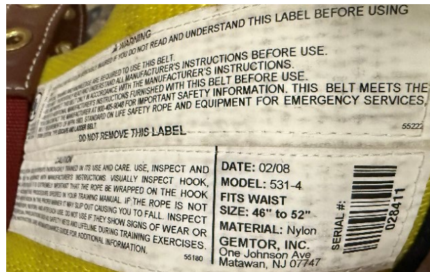
The ladder belts are expired. They need to be replaced when they are ten years old.
