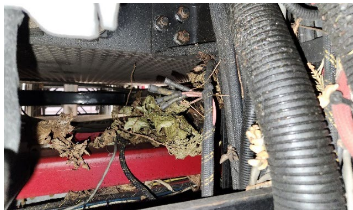
A large number of leaves and debris have caught under the underside of the apparatus, which requires thorough steam cleaning.
