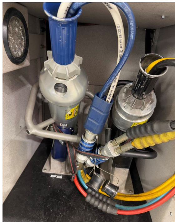
The strap does not allow for tools to be easily deployed on an incident.
