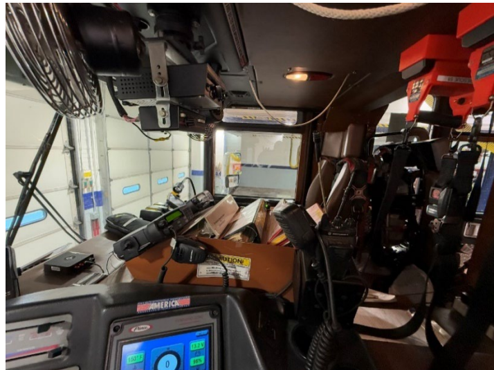
Mounting items such as fans and radios in the driver's sight line is hazardous and should be avoided.
