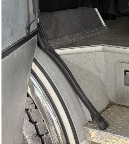
Replace or repair door rubber gaskets that are damaged.
