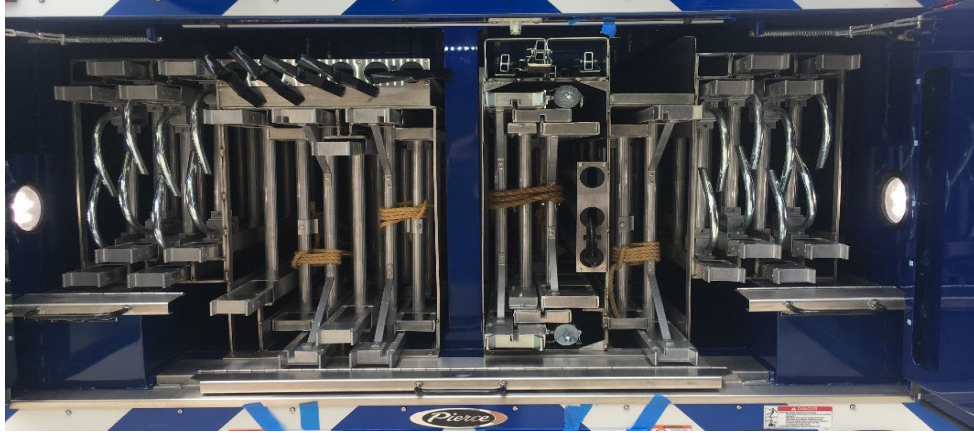
This tractor-drawn aerial ladder is equipped with 463' of ground ladders.
