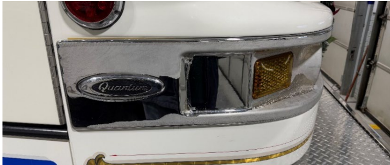
Chrome delamination needs to be addressed.
