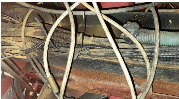
The frame rails on Engine 14-2 show their age with significant surface rust.
