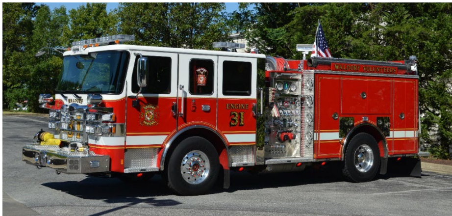
An example of a short wheelbase engine with a 750-gallon water tank.
