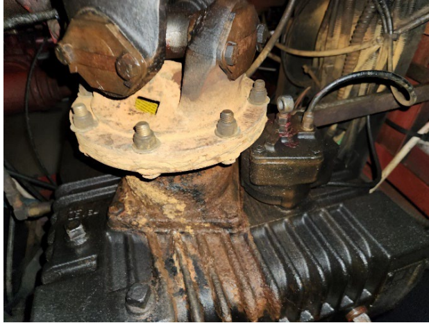
The pump packing on Engine 14-2 is leaking.
