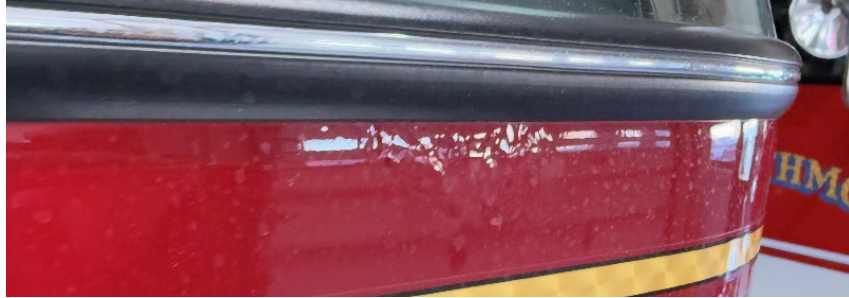
Bubbling paint and corrosion need to be mitigated under the front windshield.
