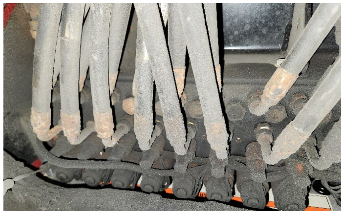
Moderate rust was noted throughout the underside of the apparatus, which needs to be mitigated.
