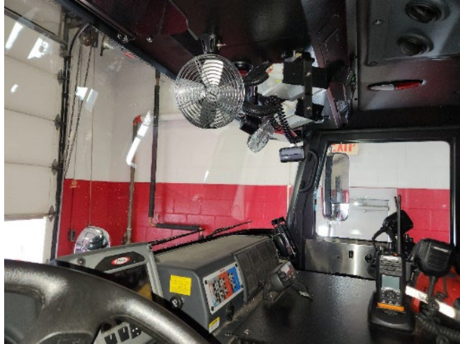
The driver's vision is partially obstructed.
