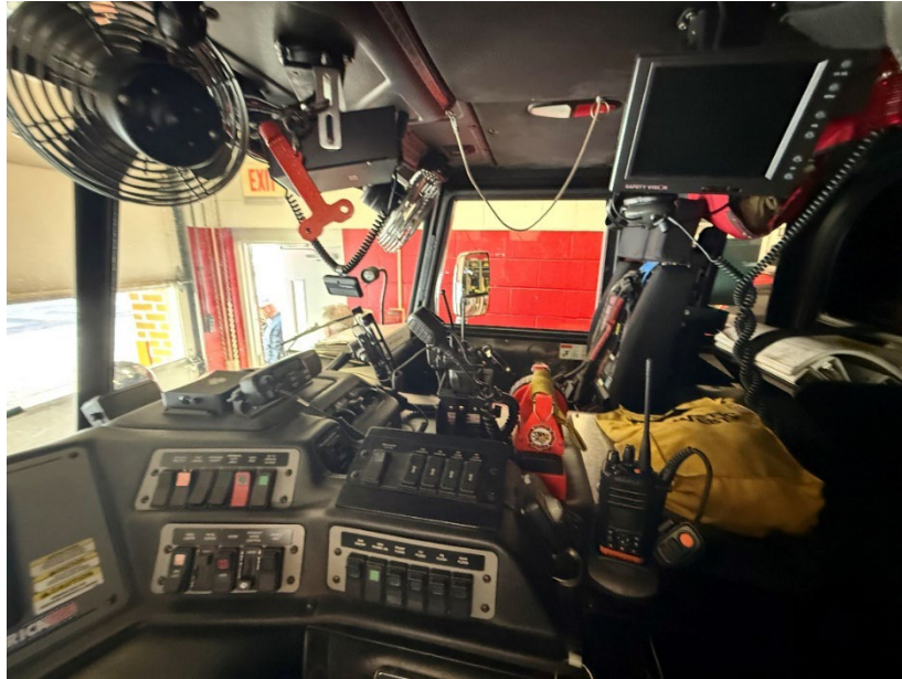
The Driver's view is badly obstructed. This needs to be mitigated in the next apparatus design.
