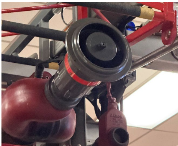
The combination nozzle should be removed and replaced with a set of stacked smoothbore tips with a stream shaper.
