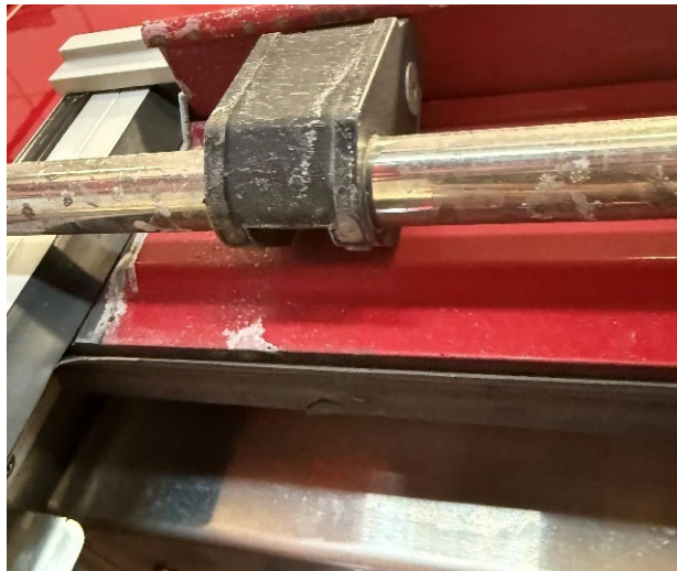
Roll-up door gaskets should be replaced to prevent dirt and moisture in the compartments.
