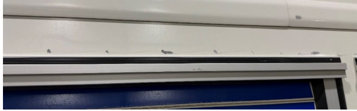
Chipped paint can allow rust to form on the body, causing damage.
