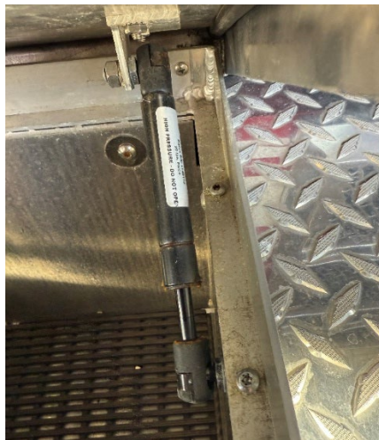
Gas Shocks on the front bumper compartment cover need to be replaced.
