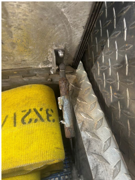
All corroded latches and corroded gas struts need to be replaced.
