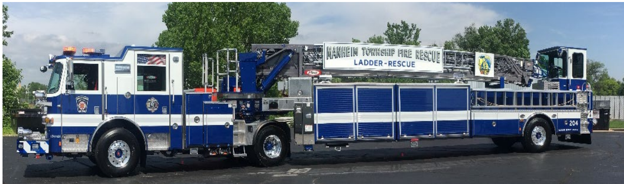
Example of a Tractor Drawn Aerial Ladder that would fit the needs of the Garden City Fire Department. The overall length is 61'3". The Garden City Station is 56 feet long, so this unit would not fit. The Shortest Tractor Aerial Ladder that EVR is aware of is 55 feet 8 inches, which still would not fit; therefore, alterations to the station would be necessary if this is the direction the fire department and the township take.
