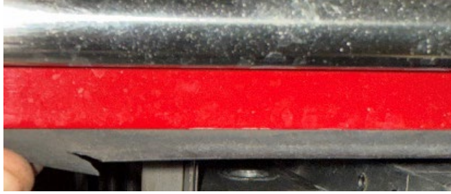
Replace the rubber gasket on the Goretite roll-up door.
